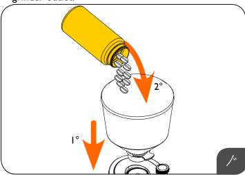
Reassemble bean hopper and fll with one cap of Grindz cleaning tablets and reopen bean stop.
