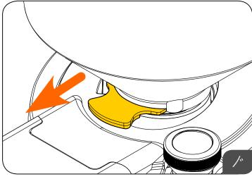
■ Connect the machine to the mains socket and pull the tab at the bottom of the hopper to open it.
