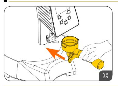
Place the flter holder onto the fork and insert it againsttheflterholderrestraint.
