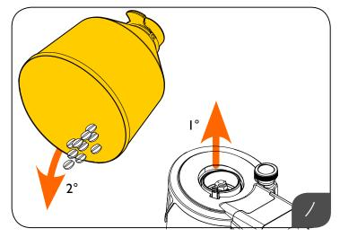
■ Turn OFF the grinder, remove the bean hopper and pour out the remaining coffee beans.
