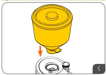
■ Insert the hopper into its seat; positioning it so that the hole lines up with the screw on the back part of grinder.
