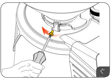
■Tighten the lock screw.
