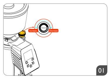
Use the grinding adjustment knob to set the grinding fneness.
